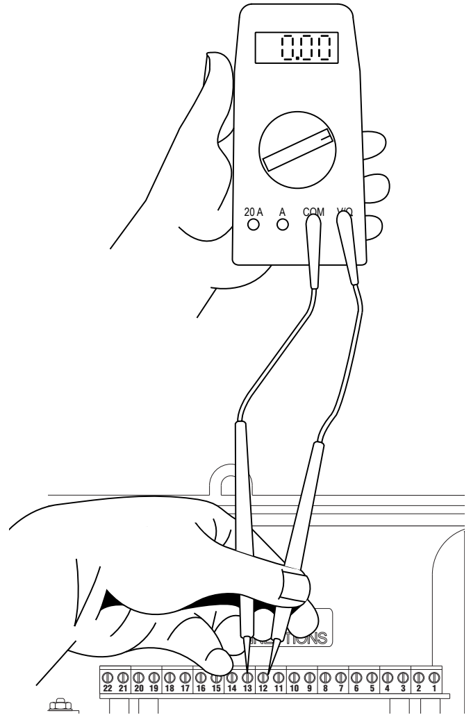
Figure 23. APS-3C/APS-4C/SC-40C Electrician's DVM Connection, Pins 12 and 13.
